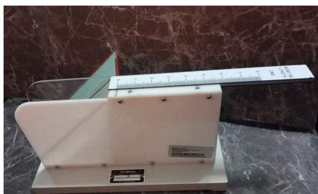
Fig. 1. The Cantilever platform for bending length tests
